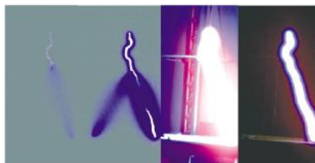
(c)左线电极 \phi 17 mm,右线电极 \phi 50 mm
